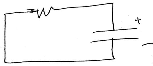
The emf has been removed from the circuit.
