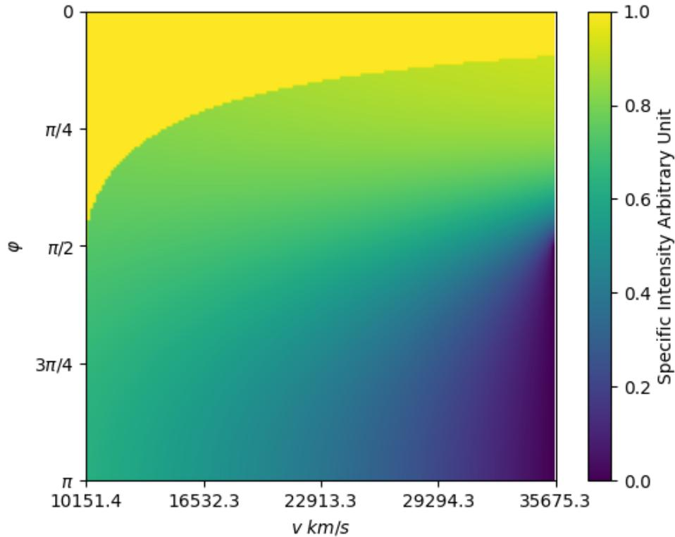
**Figure 9.** The specific intensity formal solution given in color format for our SN Ia atmosphere with specific intensity as a function of velocity coordinate and viewing angle  $\varphi$  for a single representative frequency with  $k_{\text{abs}}$  and  $j_{\text{em}}$  set to constant values. The specific intensity increases as color varies from purple to yellow.
