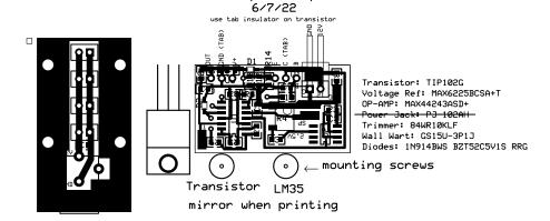
Built two like this with jumpers on R9 and D1 to match PCB to the left. The pot is also backwards (turn CCW to inc temp).
