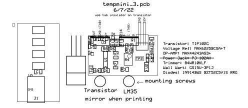
Built two like this with jumpers on R9 and D1 to match PCB to the left. The pot is also backwards (turn CCW to inc temp).
