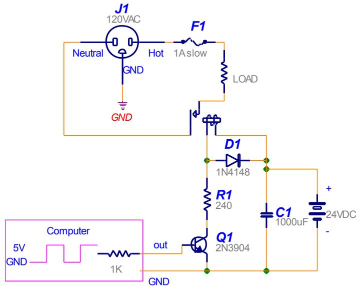
Note: R1 will get warm. Resistor power dissipation =  $12V \cdot 0.05A = 300mW$ .
