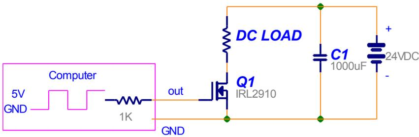
The simplest solution is to use the FET because the DC load current and voltage are less than that of the FET and the computer's output voltage and current is sufficient to fully turn on the FET. With a 5V gate drive the on resistance of the FET is 0.035Ω. This is much less than the load resistance (~12Ω if it draws 2A@24V). Because of the extremely low on-resistance a heatsink won't be needed.  $P = I^2R = (2A)^2 \cdot 0.035\Omega = 0.14W$ .
