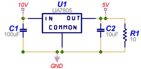
The LM7805 in the TO-220 package has the following thermal impedance:
