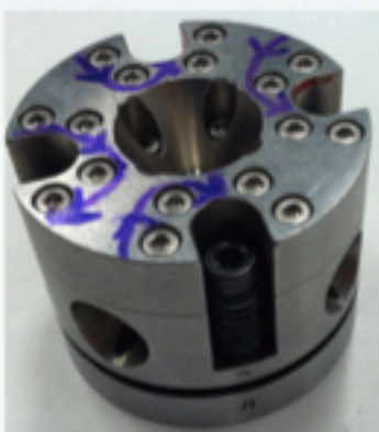
Figure 3. A view of the pressure cell that was used in this experiment.
