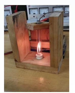
Quartz tube used to withstand temperatures
