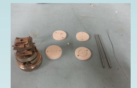
To left, 5 ceramic pieces, goniometer head, quartz tube, 2 threaded bolts and nichrome wire
