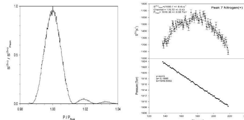
Fig. 3: Left: This plot shows the variation of the second-harmonic signal as the pressure in the cell was scanned through phase match. Right: An example of the fits used to determine peak signal and peak pressure.
