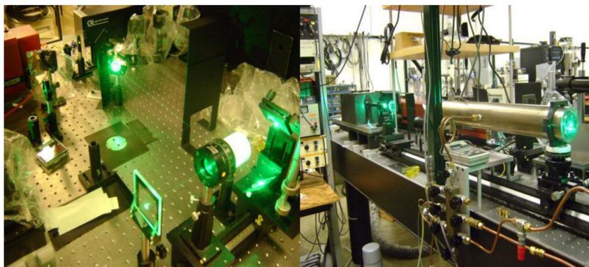
Fig. 2: Left: Upstream path of fundamental beam showing the polarizer, UV attenuator and various other optics. Right: Looking downstream: gas sample cell with the manifold and various valves used to control the pressure and composition of the cell.
