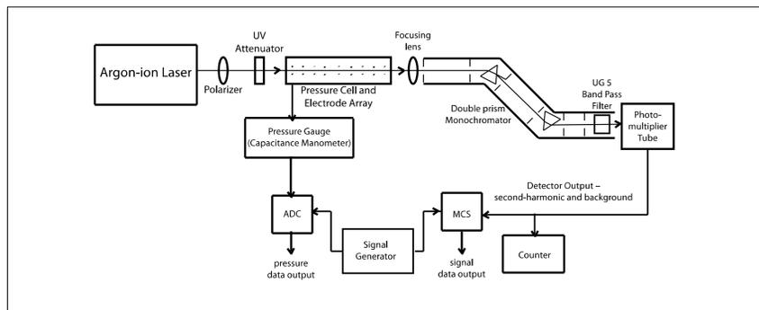
Fig. 1: Schematic diagram of the experimental apparatus, showing the cell in which the ESHG beam is produced, the monochromator which separates the second-harmonic beam, and the configuration of electronics which allows for the synchronous collection of pressure and signal data.
