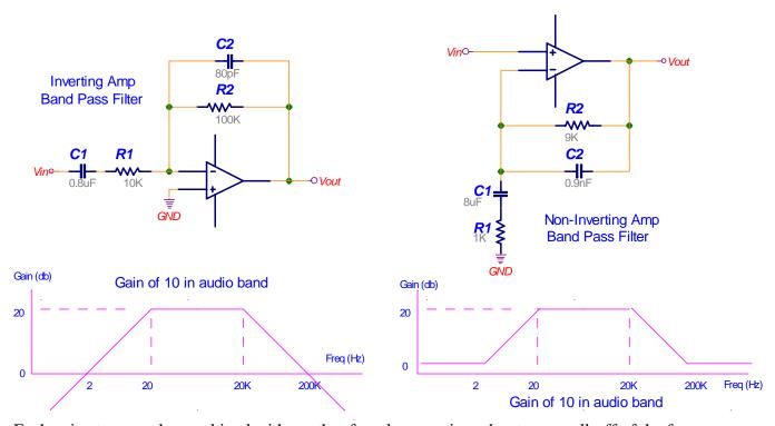
Each gain stage can be combined with another for a larger gain and a steeper roll-off of the frequency.
