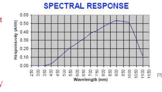
0.5uA/uW we'll need a  $2M\Omega$  feedback resistor ( $0.5A/uW*2M\Omega$  = 1V/uW). In this circuit the output voltage will go positive when light hits the photodiode. If the photodiode polarity is reversed the output would go negative when light hits the photodiode.
