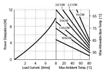
7W. If the relay's thermal resistance is given you can determine the temperature rise of the relay. The datasheet assumes you will be bolting it to a heatsink and only provides the thermal resistance between the junction and the case and not between the case and the ambient air.
