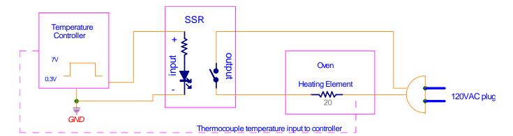
Since the load is a  $20\Omega$  resistive heater powered from the wall socked the max current will be:  $120V/20\Omega = 6A$ . You should be able to trigger the solid state relay from the controller output which is 7V at up to 20mA.
