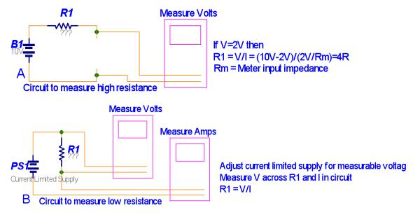
**Experiment**: Measure the resistance of the two items given to you (one is  $<< 1\Omega$  the other is  $>> 1M\Omega$ ).
