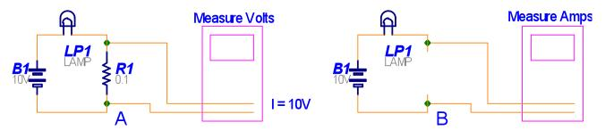
**Experiment:** Using a circuit similar to B above, determine the size of the sense resistor in the multimeter for both the <300mA and <10A settings. You may use a second voltmeter.
