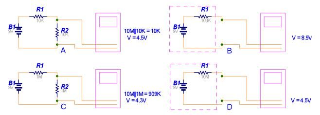
**Experiment**: Use a circuit similar to example D above to measure the input impedance of the multimeter. Adjust R1 until the measured voltage is half of the supply voltage. If the voltage drop is the same then they have to have the same impedance (i.e. the meter input impedance is the same as R1).
