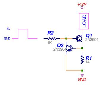
This circuit will limit the current through the load to about 50ma. As before when the input to the base resistor is 5V Q1 turns on and current flows through the load. When the input is low Q1 is off and no current flows through the load.
