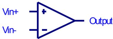
A comparator compares the voltages at the + and - inputs. If the + input is more positive than the - input the comparator output will be high. If the - input is more positive than the + input the comparator output will be low.
