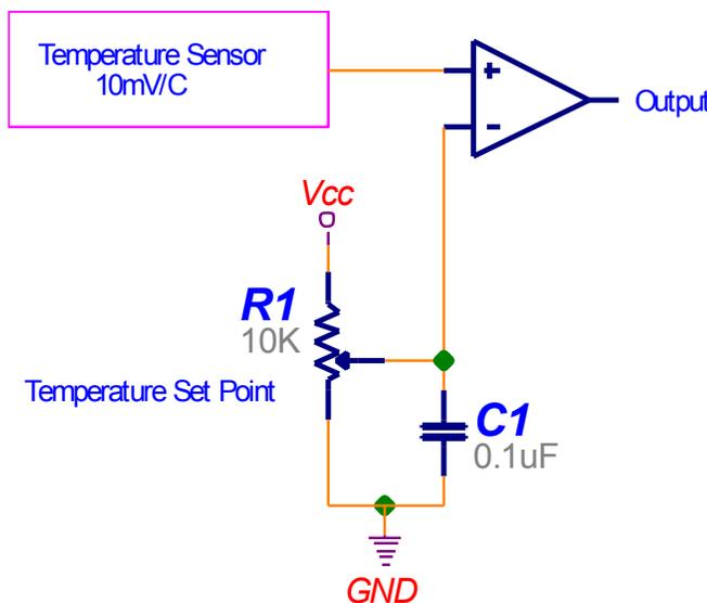
This is an example of a thermostat circuit. The temp sensor puts out 10mV/C. The pot (short for potentiometer) lets the user dial in desired temperature. The capacitor helps to short any high frequency noise on the set point voltage to ground. Note: The cap isn't needed but it's a good idea to have it.
