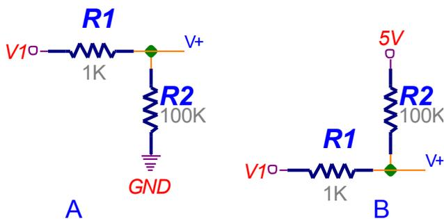
Ex: Assume V2 is 1V and V1 is 0.5V. Because V+ is less than V- the output is low. R2 feeds back some of the output voltage to the V+ input (Fig A). This makes the voltage at V+ slightly lower than V1. The larger the ratio of R2/R1 the smaller the hysteresis will be. In this case V+ will be about 1% less than V1. Because of the feedback V1 must now increase to 1.01V before V+ will reach 1V and cause the comparator output to go high. When the output goes
