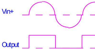
Convert a sine wave to a square wave (usually with a TTL output, i.e. a digital output, 0-5V). This can be used to make a frequency counter by sending the output into a counter and counting the number of pulses in one second.
