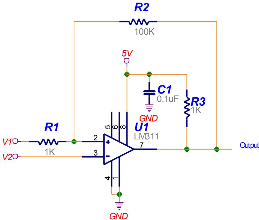
This circuit will compare two voltages, V1 & V2, and will add a little hysteresis so the output doesn't oscillate when V1 = V2. Note: Since the comparator is powered from a 0-5V supply the two input voltages should be between 0 & 5V.
