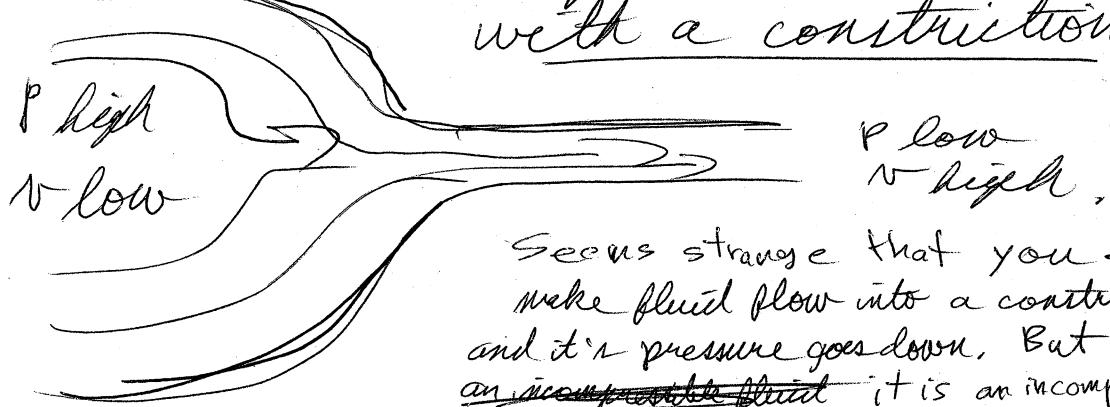
Seems strange that you ~~make~~ make fluid flow into a constriction and its pressure goes down. But ~~that's~~ ~~an incompressible fluid~~ it is an incompressible fluid and if driven thru a constriction in steady flow it <sup>decompresses</sup> by converting pressure energy to bulk kinetic energy.
