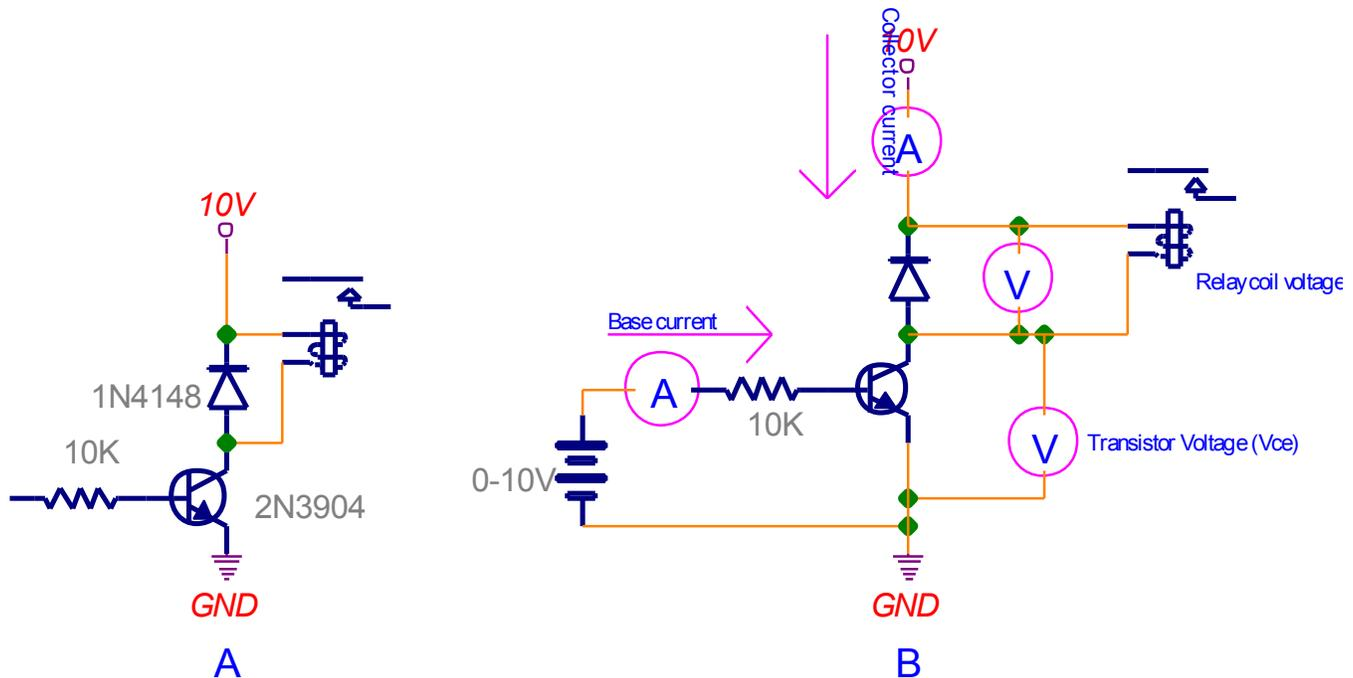
The following lists the input condition (i.e. the battery voltage) and all other voltages and currents. Note: The relay coil voltage and the transistor voltage must add up to the power supply voltage (10V in this case). We'll assume the relay coil has a DC resistance of  $50\Omega$ , the transistor has a gain ( $h_{fe}$ ) of 100, and  $V_{be} = 0.7V$  when forward biased.
