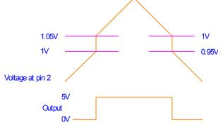
and keeps the output from oscillating. When the ramp is decreasing V1 must be 0.96V for pin 2 to reach 1V. The voltage at pin 2 jumps from 1V to 0.95V (0.96V + 1% of (0V output - 1V input)).
