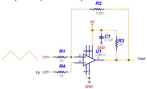
Like the demo done in class, V1 is a ramp provided by the function generator. The ramp goes between 0 & 4V. V2 is a constant 1V therefore the inverting input is a constant 1V. 1% of the difference between the input and output voltage is fed back to the positive input to keep the output from oscillating when V1 and V2 are at the same voltage.
